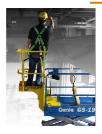
Some manufacturers now have an attachment that allows a worker on a mobile elevating work platform to be able to reach tight areas, such as in between roof trusses as the picture shows on a Genie Scissors Lift. Always refer to the manufacturers recommendations before adding any type of attachments to your work platform.
