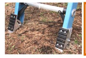
On soft ground surfaces, such as mud, rock, or gravel, rotate your ladders feet so that the rugged edges of the feet are pointing towards the ground. Push the feet into the ground to secure the ladder.
