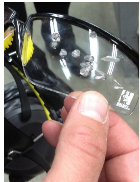
(Z-87 Safety Glasses intentionally shot with a nail gun show that eyes would have been protected.)
