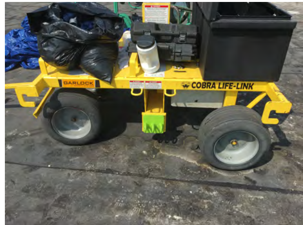
Fall Carts - Are you tied off on the correct D-Ring (Restraint V Arrest)? Is the cart parallel to the roof edge?
